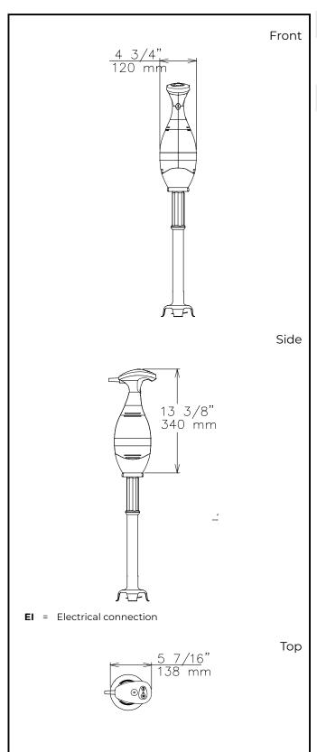
Electric Supply voltage: 110-120 V/1 ph/50/60 Hz **Total Watts:** 0.45 kW Plug type: USA NEMA 5-15P Key Information: External dimensions, 5 7/16" (138 mm) Width: External dimensions, 4 3/4" (120 mm) Depth: External dimensions, Height: 34 1/16" (865 mm) **Shipping width:** 11 7/16" (290 mm) Shipping depth: 27 3/16" (690 mm) Shipping height: 7 1/16" (180 mm) **Shipping weight:** 12 lbs (5.5 kg)
